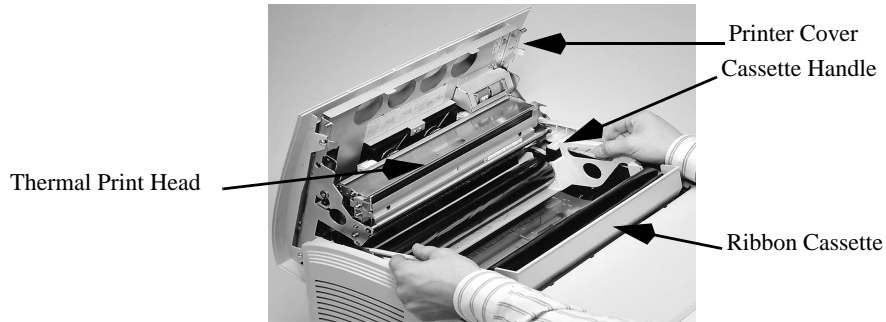
Figure 3-2 Lifting the Ribbon Cassette Up and Toward You
